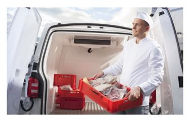
Today's compact van models offer little space for retrofitting a transport cooling systems. Quite often, it is impossible to integrate a belt-driving compressor in the engine compartment. The new generation Dometic Frigo DC systems solve this problem in a smart way. The compressor and the condenser are combined in a compact unit which is fitted in the spare wheel compartment. Like with all Dometic Frigo systems, the evaporator is mounted to the ceiling of the cargo hold.
