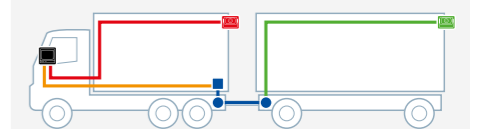
SCOPE OF ORDER: TRAILER WITH LOW COUPLING Dometic PerfectView reversing video system
