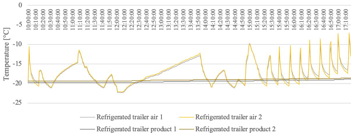
Figure 11. Sensors' measures of the temperatures inside the refrigerated vehicle and of the frozen product (Traditional refrigeration system)
